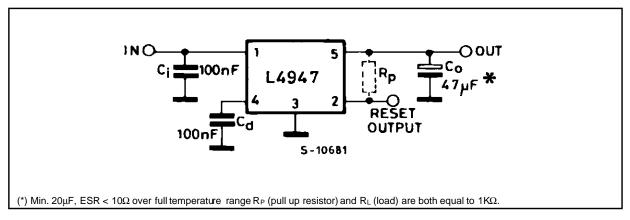
**ELECTRICAL CHARACTERISTICS** (refer to the test circuit,  $V_i = 14.4V$ ,  $C_o = 47\mu F$ , ESR <  $10\Omega$ ,  $R_p = 1K\Omega$ ,  $R_L = 1K\Omega$ ,  $-40^{\circ}C \le T_J \le 125^{\circ}C$ , unless otherwise specified)
