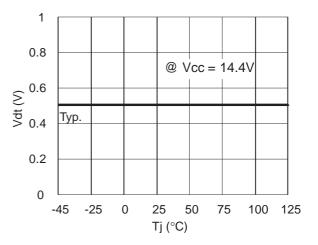
Figure 6. Dead Time vs. Temperature.
