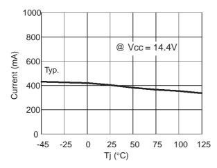
Figure 11. Output Source Current vs. Temperature.
