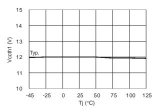
Figure 10. Vcc UV Turn Off vs. Temperature
