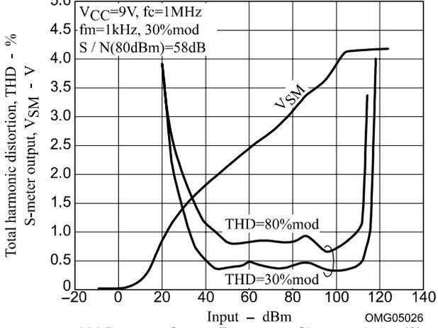
AM Detector Output Frequency Characteristics (1)
