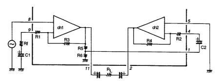
The output of ch1 is divided with R5, R6 and led to pin 1 and then inputted to ch2. Since the attenuation degree (R5/R6) of ch1 output and the amplification degree (R4/R2 + R6)) of ch2 are fixed at an equal value, the ch2 output is in opposite phase with the ch1 output. Therefore, the total voltage gain gets apparently 6 dB higher than the voltage gain of ch1 alone and is determined by the following equation.
