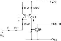
Note: Connect INR to  $V_{\mbox{\scriptsize CC}}$  when INR and OUTR are not used.
