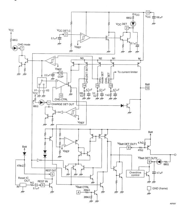
Notes: 1. Use capacitors with little temperature-related capacitance fluctuation.
