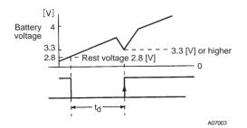
The  $V_{Batt}$  circuit operates at the edge where the reset voltage becomes Hi. (At this time, the output transistors are set on and the load is put on; If this voltage is 3.3 [V] or higher, the  $V_{Batt}$  circuit operates, and if it is lower than 3.3 [V], it does not start up.
