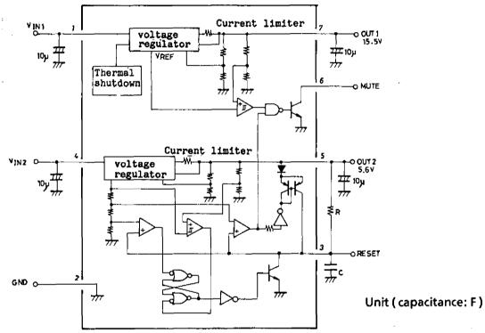
(Note) The reset delay time is set by R, C.
