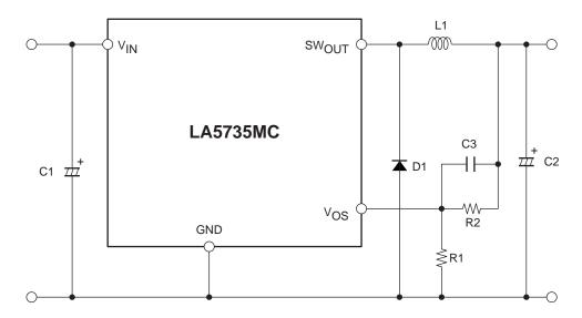
Note: Insome cases, the output may not turn on if power is applied when a load is connected. If this is a problem, increase the value of the inductor.
