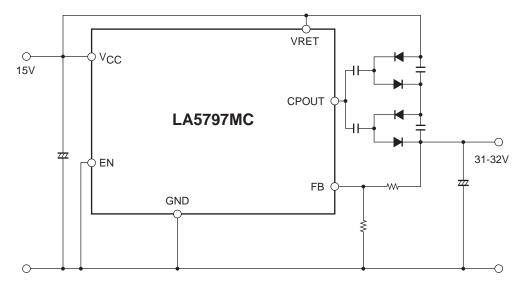
Note : The IC is made active when the EN pin is pulled down to GND. The charge pump operation is stopped when the EN pin is pulled up to  $V_{\mbox{IN}}$ .
