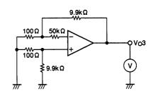
$$\cdot I_{B} = \frac{|V_{O}3 - V_{O}1|}{50k \times 100}$$
