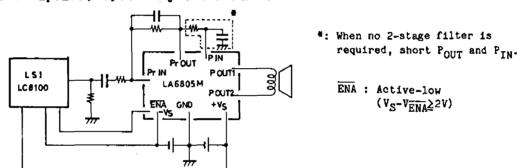
(2) Application where the LA6805M is used in conjunction with the current output type (bipolar) speech synthesis LSI.
