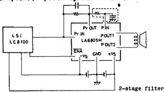
(3) Application where the LA6805M is operated from a single supply
