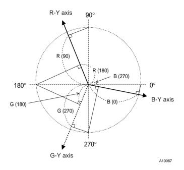
8. The method for calculating the AF angle is shown below. BR · · · · The B-Y/R-Y demodulation output ratio  $\theta$ · · · · · · ANGBR: the B-Y/R-Y demodulation angle
