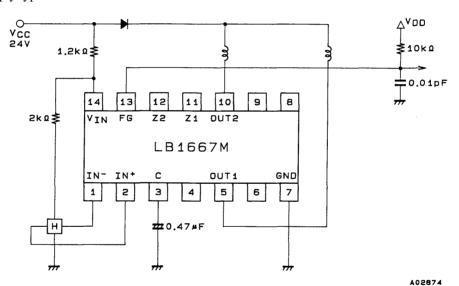
• Circuit for use when large output currents are required and heat dissipation is high.
