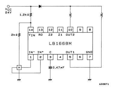
• Circuit for use when large output currents are required and heat dissipation is high.
