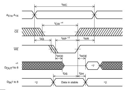
[Write cycle 2] ( $\overline{\text{CE}}$  write) \*6
