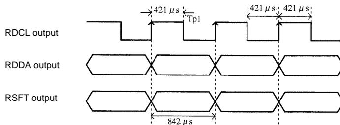
Note: When PT2 = 0, RDDA and RSFT must be acquired on the falling edge of RDCL.
