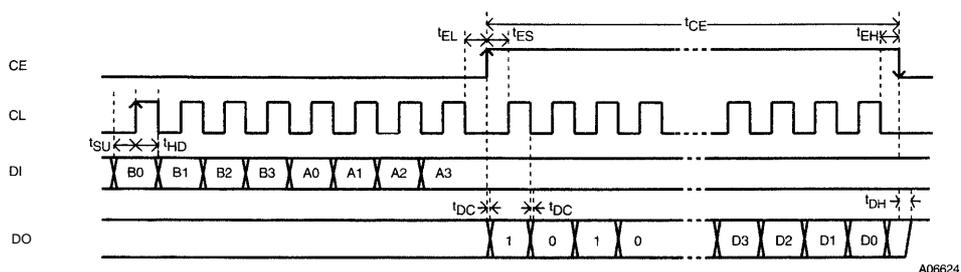
Notes: 1. Since the DO pin is an n-channel open-drain output, the transition times ( $t_{DC}$ ,  $t_{DH}$ ) will differ with the value of the pull-up resistor used.
