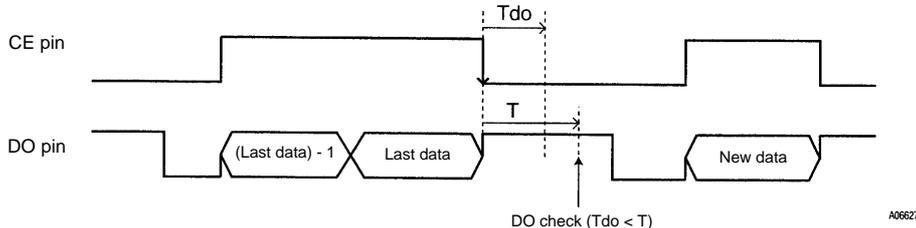
2. When the DO pin is low following the  $265 \mu s$  period ( $T_{do}$ ) after data is read out
