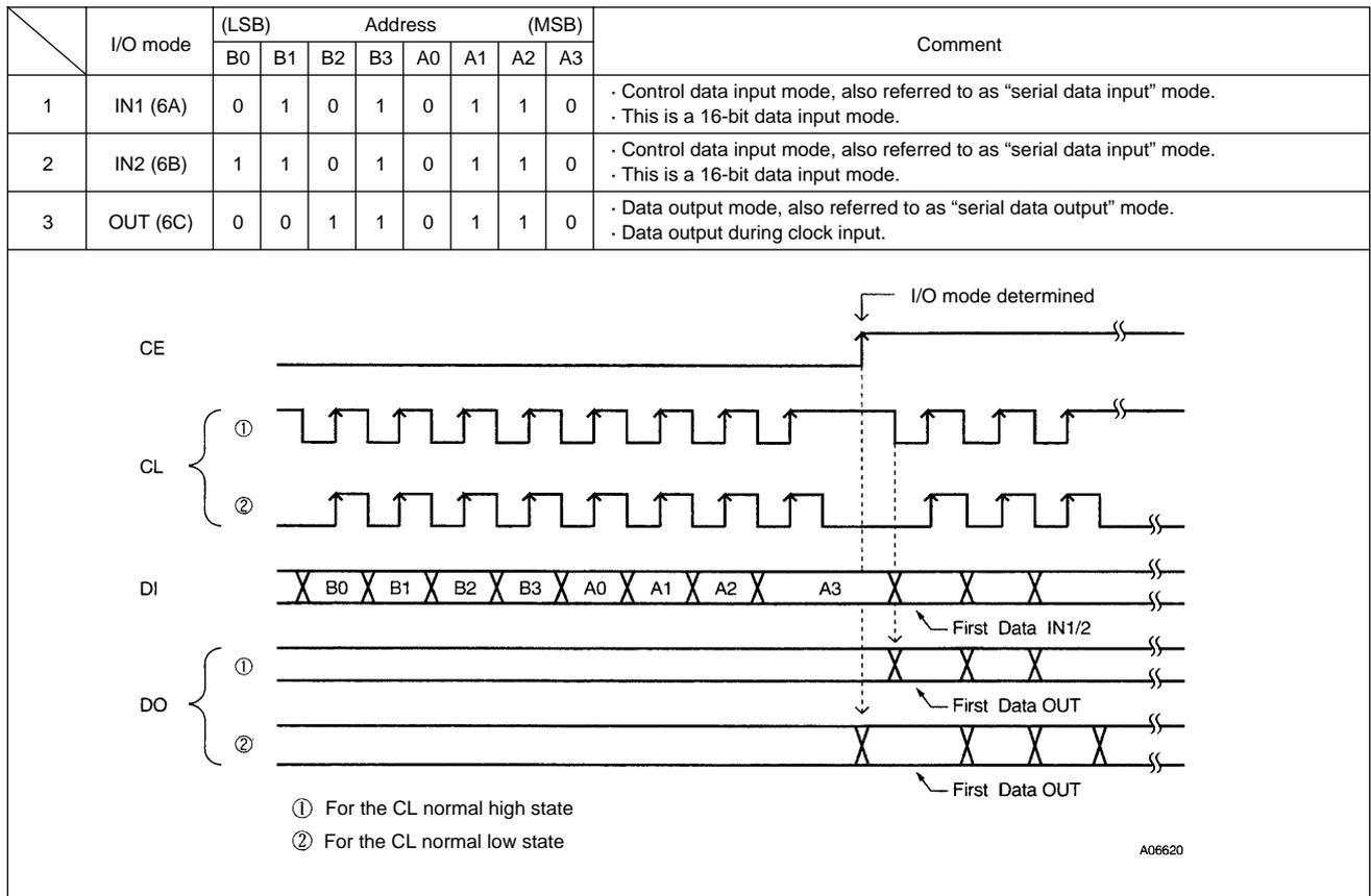
**Serial data input (IN1, IN2)**  $t_{SU}, t_{HD}, t_{EL}, t_{ES}, t_{EH} \geq 0.75 \mu s$   $t_{LC} < 1.15 \mu s$   $t_{CE} < 20 ms$
