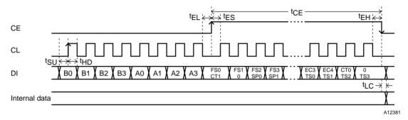
$\textbf{Serial data output (OUT)} \ t_{SU}, \ t_{HD}, \ t_{EL}, \ t_{ES}, \ t_{EH} \geq 0.75 \ \mu s \ \ t_{DC}, \ t_{DH} < 0.46 \ \mu s \ \ t_{CE} < 20 \ ms$
