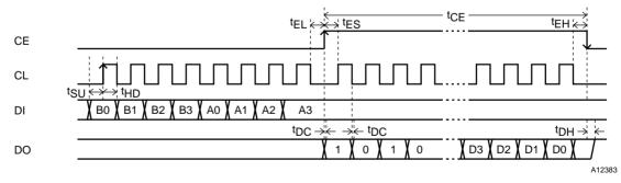
Notes: 1. Since the DO pin is an n-channel open-drain output, the transition times  $(t_{DC}, t_{DH})$  will differ with the value of the pull-up resistor used.
