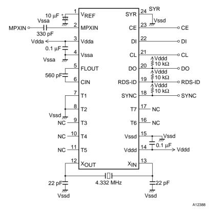
Notes: 1. Determine the value of the DO pin pull-up resistor based on the required serial data transfer speed.
