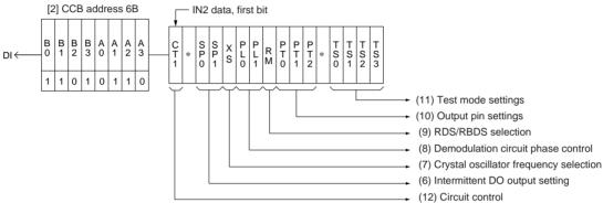
Caution: The bits labeled with an asterisk must be set to 0.
