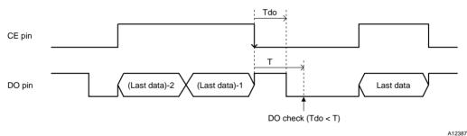
Notes: 1. Although an application can determine whether or not there is data remaining in the buffer by checking the DO level with the above timing, checking the RE and RF flags in the serial data is a preferable method.
