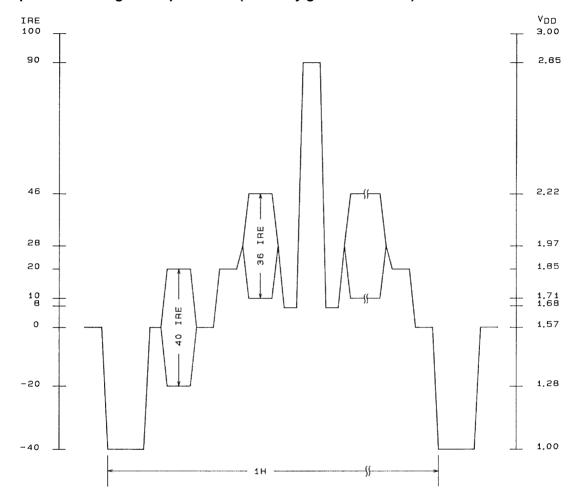
Composite Video Signal Output Levels (internally generated levels)
