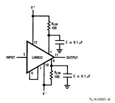
FIGURE 3. LH0033 Using Resistor Current Limiting
