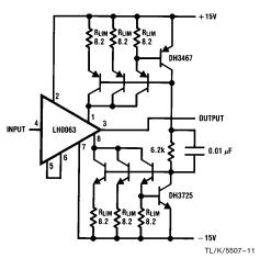
FIGURE 6. LH0063 Current Limiting Using Current Sources
