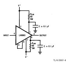
FIGURE 4. LH0063 Using Resistor Current Limiting
