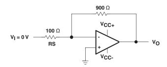
Figure 2. Noise-Test Circuit
