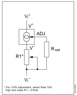
Figure 4: Zero Temperature Coefficient Current Source
