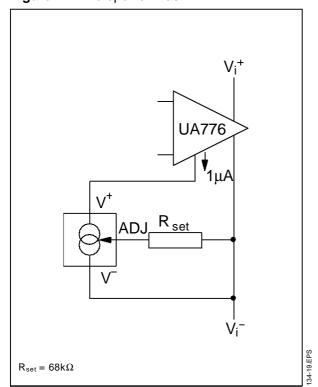
Figure 6: Low Output Impedance Thermometer
