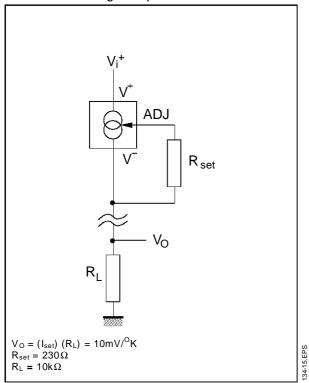
Figure 2: Alternate Trimming Technique
