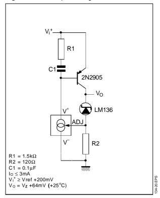
Figure 9: In-line Current Limiter
