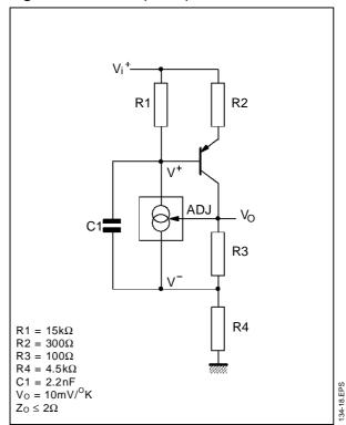
Figure 8: Low Input Voltage Reference Driver
