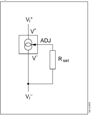
Figure 3: Terminating Remote Sensor for Voltage Output
