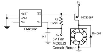
The LM26NV switches the fan on when the measured temperature exceeds the trip temperature.
