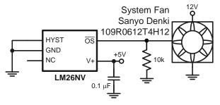
The fan's control pin has an internal pull-up. The 10 kOhm pull-down sets a slow fan speed. When the output of the LM26NV goes low, the fan will speed up.
