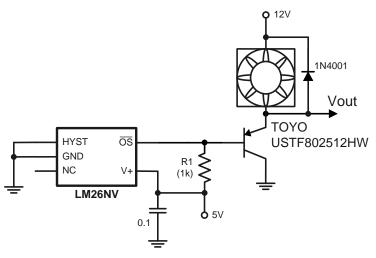
The LM26LV sinks causes the switch to sink the fan current when the measured temperature exceeds the trip temperature.
