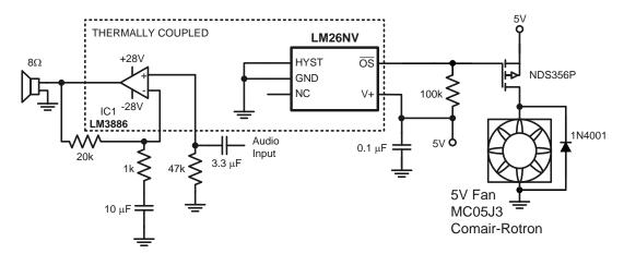
By thermally coupling the LM26NV to the audio power amplifier, the LM26NV safeguards the amplifier from overheating, turning on the fan when it temperature exceeds the trip temperature.
