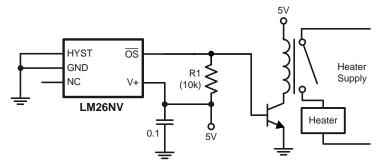
When the measured temperature is below the trip temperature of the LM26NV, the  $\overline{OS}$  output will be high, causing the switch and relay to close. When the temperature exceeds the trip point,  $\overline{OS}$  goes low and shuts off the relay and heater.
