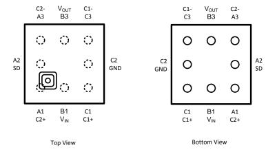
Figure 1. 8-Bump Thin DSBGA Package
