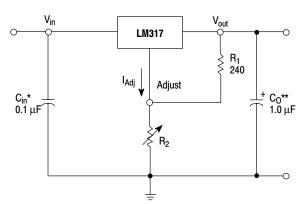
\*  $C_{in}$  is required if regulator is located an appreciable distance from power supply filter. \*\*  $C_O$  is not needed for stability, however, it does improve transient response.
