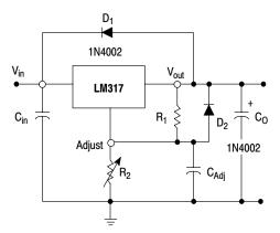
Figure 18. Voltage Regulator with Protection Diodes
