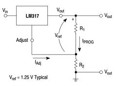
Figure 17. Basic Circuit Configuration
