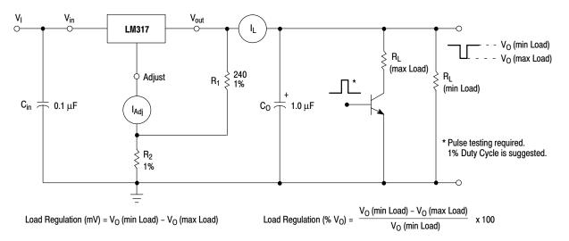
Figure 2. Load Regulation and  ${\scriptstyle \Delta I_{Adj}}\!/\!\text{Load}$  Test Circuit
