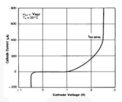
Figure 6. Cathode Current vs. Cathode Voltage
