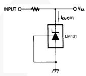
Figure 4. Test Circuit for I<sub>KA(OFF)</sub>
