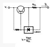
Figure 15. Current Limit or Current Source
