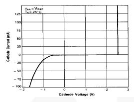
Figure 5. Cathode Current vs. Cathode Voltage
