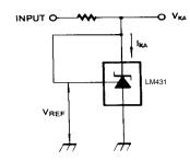
Figure 2. Test Circuit for  $V_{KA} = V_{REF}$
