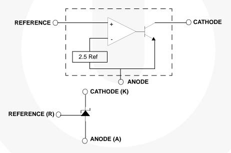
Figure 1. Block Diagram
