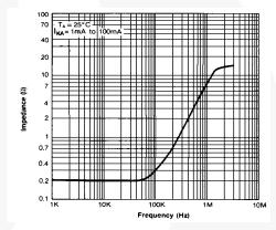
Figure 8. Dynamic Impedance Frequency
