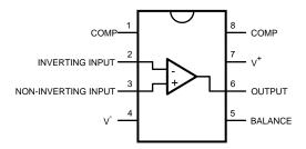
Figure 1. Dual-In-Line Package - Top View
