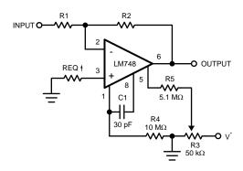
†May be zero or equal to parallel combination of R1 and R2 for minimum offset.
