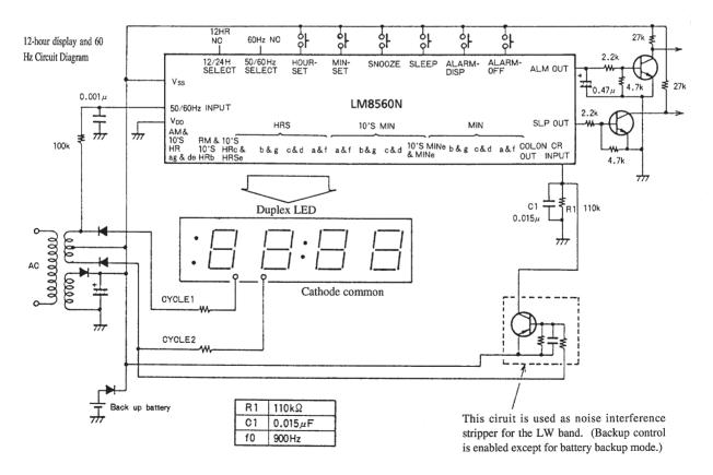
Unit (resistance:  $\Omega$ , capacitance: F)
