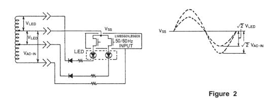
$V_{AC-IN}$  represents the average value for input voltage of the 50/60 Hz input pin.  $V_{LED}$  represents the average value for power supply voltage for LED usage.
