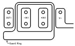
TL/H/11423-€ FIGURE 3. Example of Guard Ring in P.C. Board Layout
