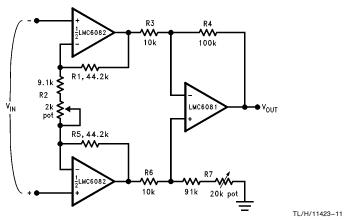
If  $R_1 = R_5$ ,  $R_3 = R_6$ , and  $R_4 = R_7$ ; then
