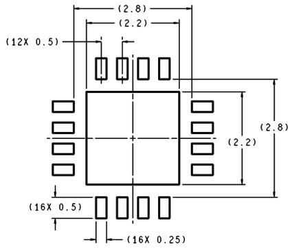
DIMENSIONS ARE IN MILLIMETERS
