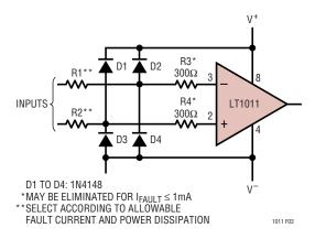
Figure 3. Limiting Fault Input Currents
