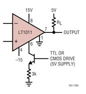
Figure 4. Typical Strobe Circuit
