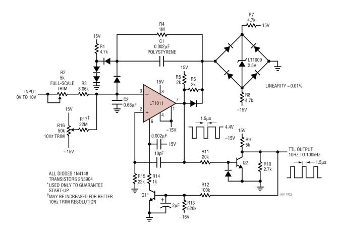
10Hz to 100kHz Voltage to Frequency Converter
