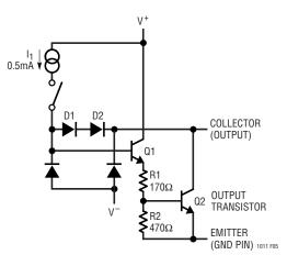
Figure 5. Output Transistor Circuitry
