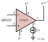
\*INPUT POLARITY IS REVERSED WHEN USING PIN 1 AS OUTPUT \*\*V^+\* MAY BE ANY VOLTAGE ABOVE V<sup>-</sup>. PIN 1 SWINGS TO WITHIN  $\approx$  2V OF V<sup>++</sup>
