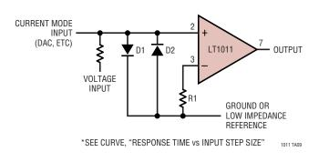
Using Clamp Diodes to Improve Frequency Response\*
