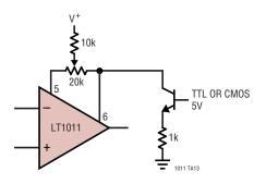
Direct Strobe Drive When CMOS\* Logic Uses Same V\* Supply as LT1011
