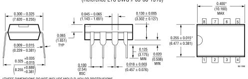
\*THESE DIMENSIONS DO NOT INCLUDE MOLD FLASH OR PROTRUSIONS. MOLD FLASH OR PROTRUSIONS SHALL NOT EXCEED 0.010 INCH (0.254mm)
