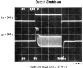
1MHz SINE WAVE GATED OFF WITH SHUTDOWN PIN,  $A_V$  = 3,  $R_{FB}$  = 1k,  $R_G$  = 500  $\Omega$
