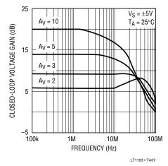
**Closed-Loop Voltage Gain vs Frequency**
