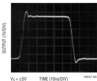
$V_S = \pm 5V$  $V_{1N} = \pm 1.25V$  $R_F = R_G = 255\Omega$   $R_L = 100\Omega$
