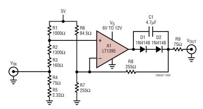
Figure 6. Single Supply RGB Video Amplifier (1 of 4 Channels)
