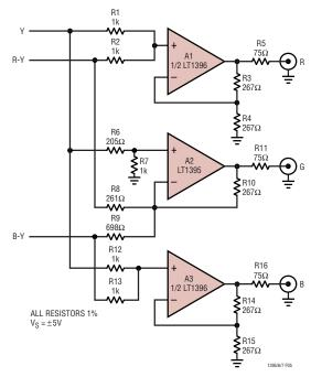
Figure 5. Buffered Color-Difference to RGB Matrix
