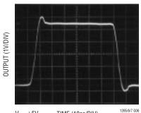
$V_S = \pm 5V$ TIME (10ns/DIV)  $V_{IN} = \pm 2.5V$  $R_F = R_G = 280\Omega$   $R_L = 100\Omega$
