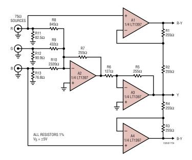
Figure 4. Buffered RGB to Color-Difference Matrix
