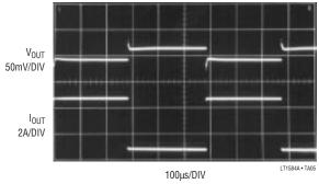
\* TRANSIENT RESPONSE MEASURED WITH AN INTEL POWER VALIDATOR. V<sub>OUT</sub> IS MEASURED AT THE POWER VALIDATOR
