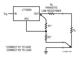
Figure 5. Connection for Best Load Regulation
