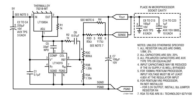
Guaranteed LT1585A Circuit for the Intel 100MHz and Higher Frequency Pentium Processors (Meets Intel Specifications with Worst-Case Tolerances)
