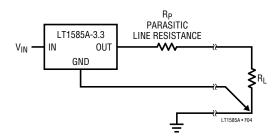
Figure 4. Connection for Best Load Regulation
