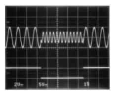
$V_S$  = 5V  $V_{IN1}$  = 1.2kHz AT 4V<sub>P-P</sub>,  $V_{IN2}$  = 2.4kHz AT 2V<sub>P-P</sub> INPUT SELECT = 120Hz AT 5V<sub>P-P</sub>
