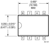
\*THESE DIMENSIONS DO NOT INCLUDE MOLD FLASH OR PROTRUSIONS. MOLD FLASH OR PROTRUSIONS SHALL NOT EXCEED 0.010 INCH (0.254mm)
