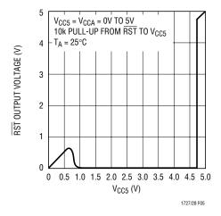
Figure 5. RST Output Voltage Characteristics of the Circuit in Figure 4
