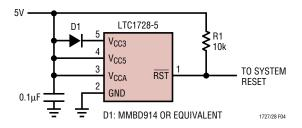
Figure 4. LTC1728-5 Monitoring a Single 5V Supply. D1 Used to Avoid RST High Near 3.1V to 4V (See Figure 3).
