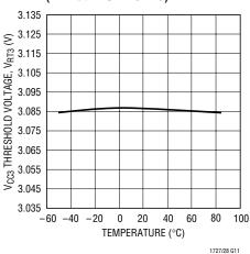
V<sub>CC5</sub> Threshold Voltage vs Temperature (LTC1727-5/LTC1728-5)
