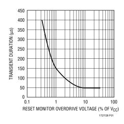
Figure 1. Transient Duration vs Comparator Overdrive
