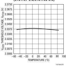
V<sub>CC3</sub> Threshold Voltage vs Temperature (All But LTC1728-1.8)
