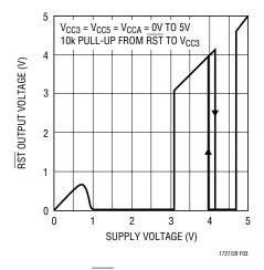
Figure 3. RST Voltage vs Supply Voltage
