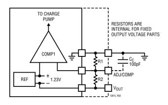
Figure 2. Regulator Loop Compensation
