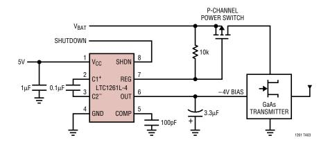
1mV Ripple, 5V Input, -4V Output GaAs FET Bias Generator
