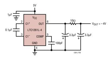
Figure 3. Output Filter Cuts Ripple Below 3mV
