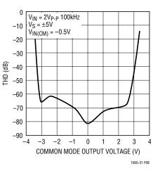
Figure 8. THD vs Common Mode Output Voltage
