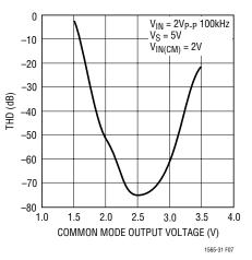
Figure 7. THD vs Common Mode Output Voltage
