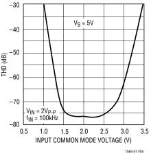
Figure 4. THD vs Common Mode Input Voltage
