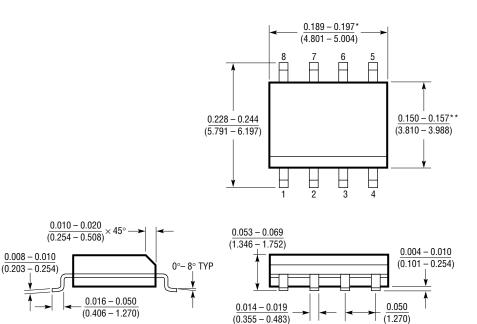
TYP \*DIMENSION DOES NOT INCLUDE MOLD FLASH. MOLD FLASH SHALL NOT EXCEED 0.006" (0.152mm) PER SIDE \*\*DIMENSION DOES NOT INCLUDE INTERLEAD FLASH. INTERLEAD
