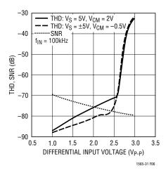
Figure 6. THD vs V<sub>IN</sub> for a Common Mode Input Voltage 0.5V Below Mid Supply
