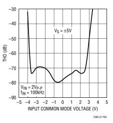
Figure 3. THD vs Common Mode Input Voltage
