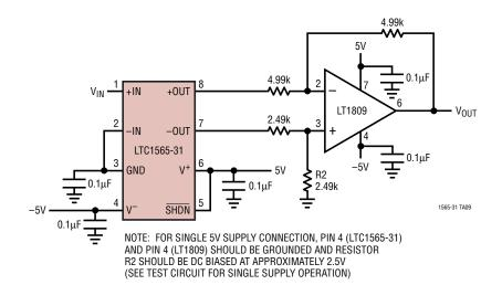
A Fully Differential Filter with Adjustable Output Common Mode Voltage
