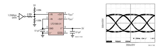
Simple Pulse Shaping Circuit for Single 5V Operation, 1.25Mbps 2 Level Data
