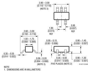
2. DIMENSIONS ARE INCLUSIVE OF PLATING 3. DIMENSIONS ARE EXCLUSIVE OF MOLD FLASH AND METAL BURR
