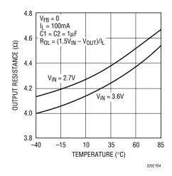
Figure 4. Typical  $R_{OL}$  vs Temperature
