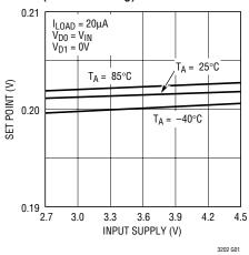
V<sub>FB</sub> Set Point vs Input Supply (600mV Setting)
