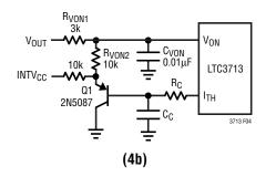
Figure 4. Adjusting Frequency Shift with Load Current Changes
