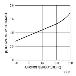
Figure 3. R<sub>DS(ON)</sub> vs Temperature
