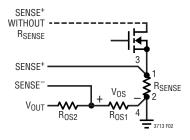
Figure 2. Sense Voltage Offset
