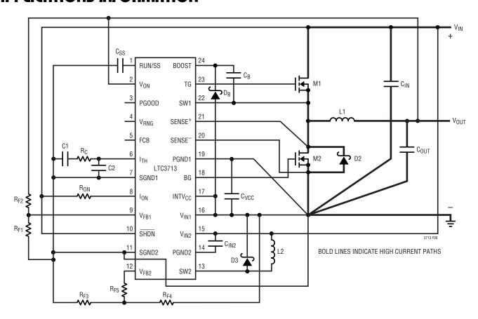
Figure 8. LTC3713 Layout Diagram
