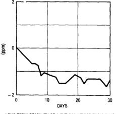
LONG TERM STABILITY OF A TYPICAL DEVICE FROM TIME = 0
