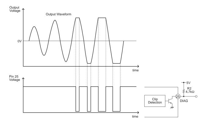
Fig3 Self-diagnosis Function Diagram
