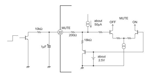
Fig2 Mute equivalent circuit
