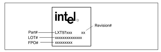
The silicon stepping in the LXT974/975 Data Sheet is referred to as "Manufacturer's Revision Number." The silicon stepping number may be read by software from Register 3, bits 3:0 in the LXT974/975 transceiver.
