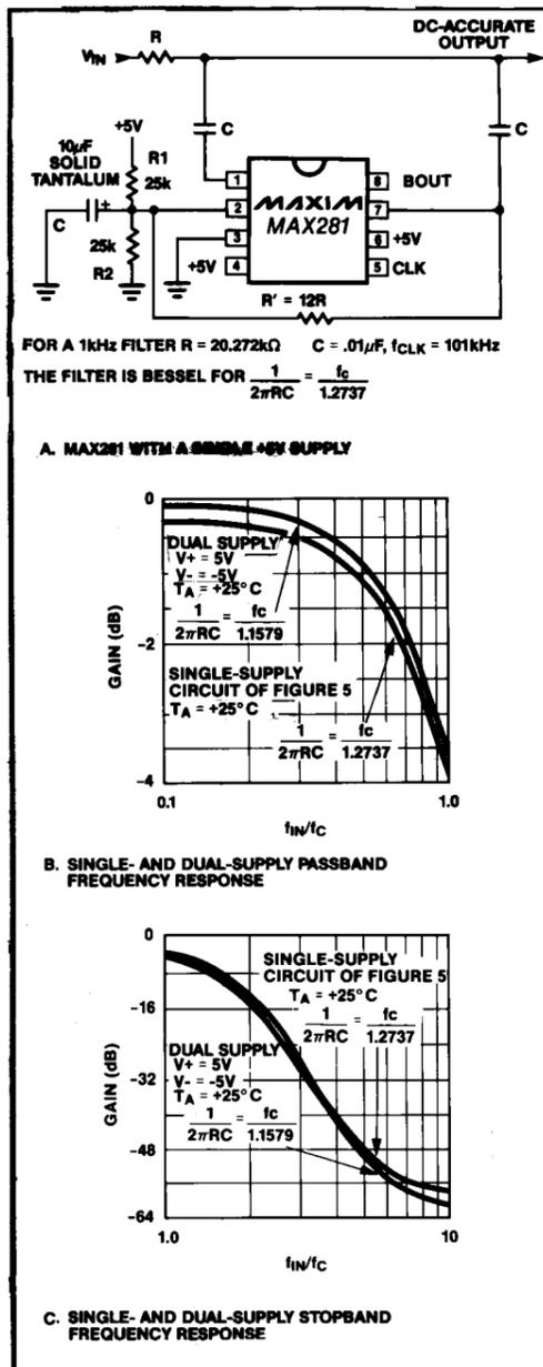
Figure 5. Operation from a Single +5V Supply
