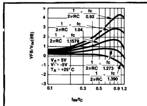
Figure 3. Amplitude Response of FB Pin
