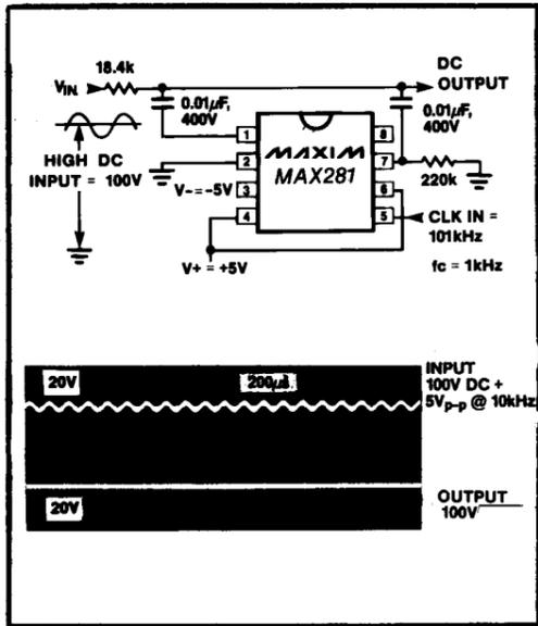
Figure 7. Filtering AC Signals from High DC Voltages
