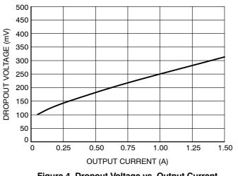
Figure 4. Dropout Voltage vs. Output Current (V<sub>OUTnom</sub> = 2.5 V)
