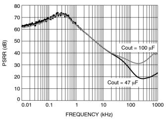
Figure 18. PSRR vs. Frequency, Vin = 3.5 V + 200 mVpp Modulation, Vout = 2.5 V, lout = 1.5 A
