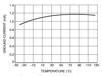
Figure 13. Ground Current vs. Temperature ( $V_{OUTnom}$  = 2.5 V,  $I_{OUT}$  = 10 mA,  $V_{IN}$  = 3.5 V)
