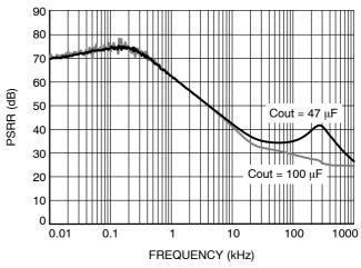
Figure 17. PSRR vs. Frequency, Vin = 3.5 V + 200 mVpp Modulation, Vout = 2.5 V, lout = 0.5 A
