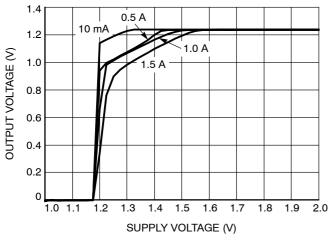
Figure 6. Dropout Characteristics (V<sub>OUTnom</sub> = 1.24 V)
