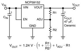
Figure 23. Adjustable Voltage Operation
