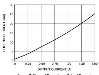
Figure 8. Ground Current vs. Output Current (V<sub>OUTnom</sub> = 1.24 V)
