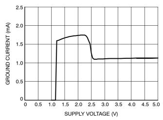
Figure 11. Ground Current vs. Supply Voltage (V<sub>OUTnom</sub> = 2.5 V, I<sub>OUT</sub> = 10 mA)
