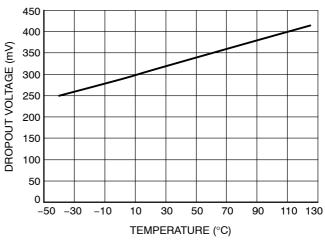
Figure 5. Dropout Voltage vs. Temperature (V<sub>OUTnom</sub> = 2.5 V, I<sub>OUT</sub> = 1.5 A)
