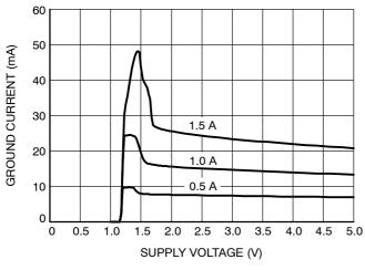
Figure 10. Ground Current vs. Supply Voltage (V<sub>OUTnom</sub> = 1.24 V)
