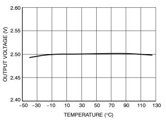
Figure 16. Output Voltage vs. Temperature (V<sub>OUTnom</sub> = 2.5 V, I<sub>OUT</sub> = 10 mA)
