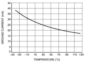
Figure 15. Ground Current vs. Temperature (V<sub>OUTnom</sub> = 2.5 V, I<sub>OUT</sub> = 1.5 A, V<sub>IN</sub> = 3.5 V)
