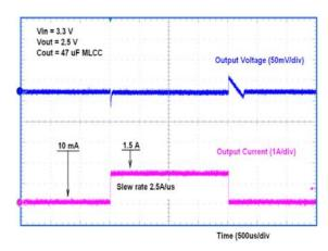
Figure 22. Load Transient Response
