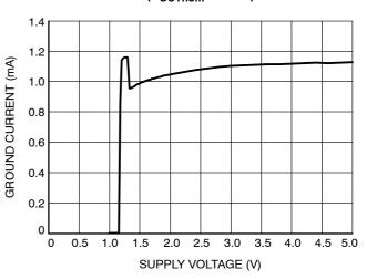
Figure 9. Ground Current vs. Supply Voltage (V<sub>OUTnom</sub> = 1.24 V, I<sub>OUT</sub> = 10 mA)
