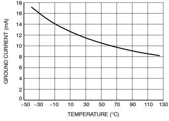
Figure 14. Ground Current vs. Temperature (V<sub>OUTnom</sub> = 2.5 V, I<sub>OUT</sub> = 0.75 A, V<sub>IN</sub> = 3.5 V)
