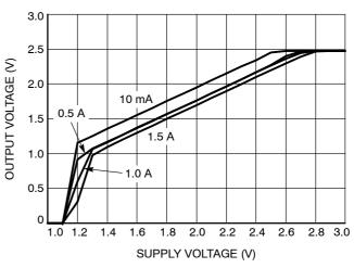
Figure 7. Dropout Characteristics (V<sub>OUTnom</sub> = 2.5 V)
