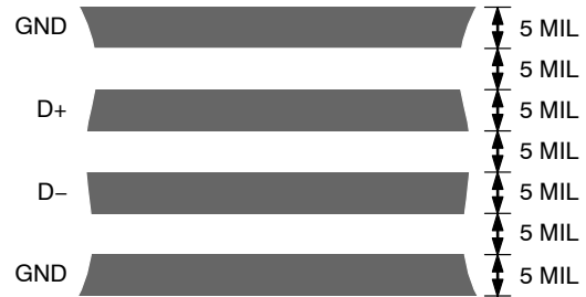
Figure 4. Typical Arrangement of Signal Tracks
