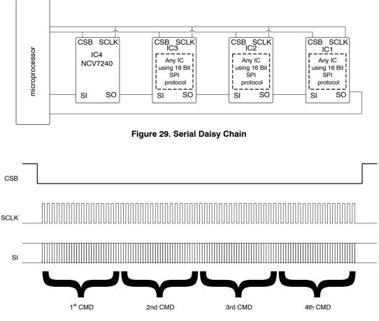
Figure 30. Serial Daisy Chain Timing Diagram
