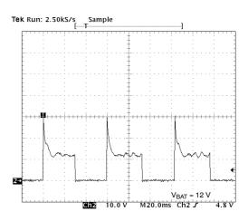
Figure 35. Typical Stepper Motor Waveform (Unipolar Portescap 35L048L32U)
