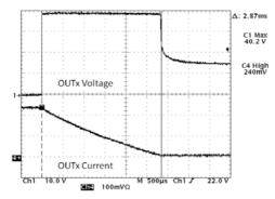
Figure 4. Repetitive Clamping Energy Test
