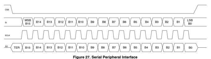
The timing diagram highlighted in Figure 27 shows the SPI interface communication. Note:
