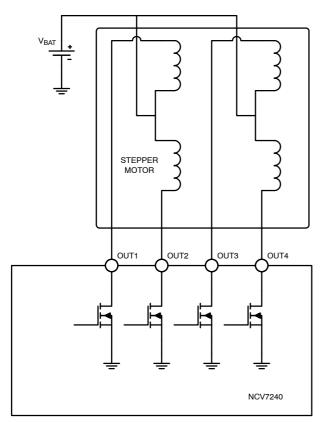
Figure 34. Stepper Motor Operation Setup
