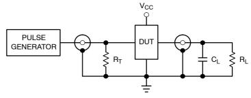
$R_T$  =  $C_L$  or equivalent (includes jog and probe capacitance)  $R_T$  =  $Z_{OUT}$  of pulse generator (typically 50  $\Omega)$
