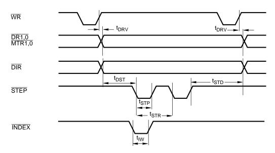
FIGURE 14-19. Drive Control Timing
