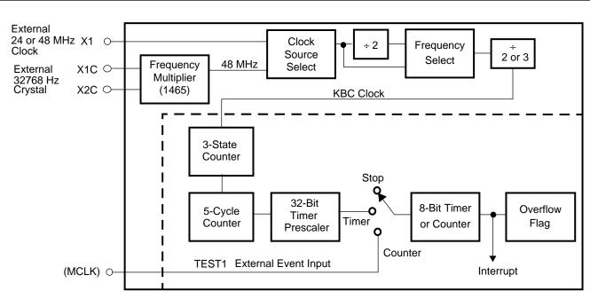
FIGURE 3-5. Timing Generation and Timer Circuit
