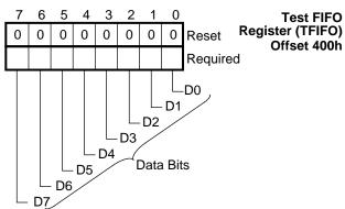
FIGURE 6-23. TFIFO Register Bitmap
