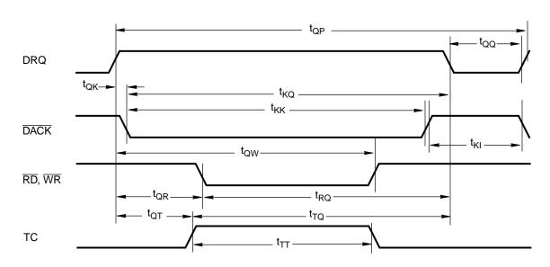
FIGURE 14-14. FDC DMA Timing
