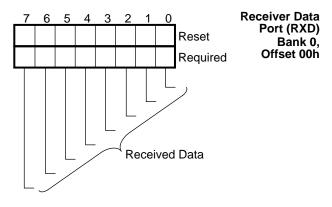
FIGURE 8-3. RXD Register Bitmap
