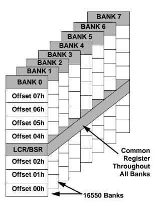
FIGURE 7-1. Register Bank Architecture
