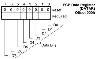
FIGURE 6-17. EPP DATAR Register Bitmap
