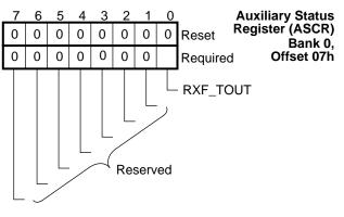
FIGURE 8-17. ASCR Register Bitmap
