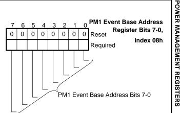
FIGURE 10-11. PM1 Bits 7-0 Register Bitmap
