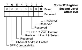
FIGURE 6-31. Control2 Register Bitmap
