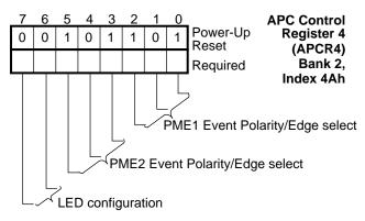
FIGURE 4-24. APCR4 Register Bitmap
