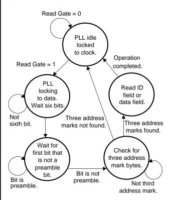
FIGURE 5-3. Read Algorithm State Diagram
