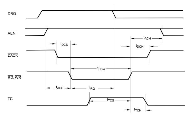
FIGURE 14-16. UART2 DMA Timing
