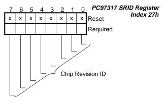
FIGURE 2-8. PC97317 SRID Register Bitmap
