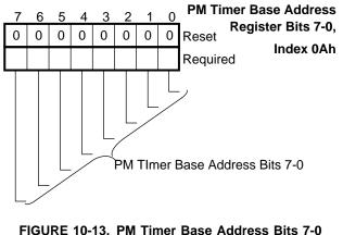
FIGURE 10-13. PM Timer Base Address Bits 7-0 Register Bitmap
