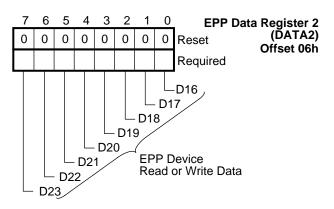
FIGURE 6-10. EPP DATA2 Register Bitmap
