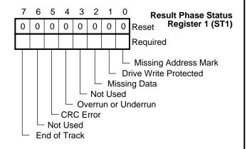
FIGURE 5-16. ST1 Result Phase Register Bitmap
