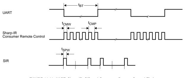
FIGURE 14-11. UART, Sharp-IR, SIR and Consumer Remote Control Timing
