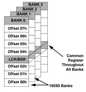
FIGURE 8-1. Register Bank Architecture
