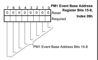
FIGURE 10-12. PM1 Bits 15-8 Register Bitmap
