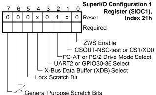
FIGURE 2-3. SIOC1 Register Bitmap
