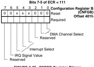
FIGURE 6-25. CNFGB Register Bitmap
