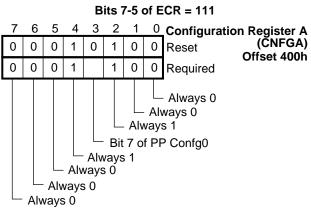
FIGURE 6-24. CNFGA Register Bitmap
