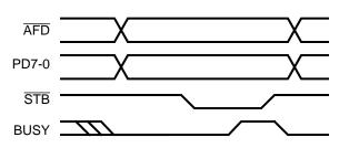
FIGURE 6-34. ECP Forward Write Cycle
