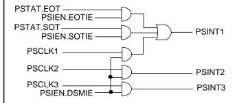
Figure 12-2. PS/2 Interface Interrupt Signals
