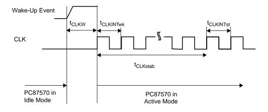
Figure 19-7. Internal Clock Generator
