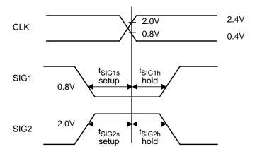
Figure 19-3. TTL: Input Signals Specification Standard
