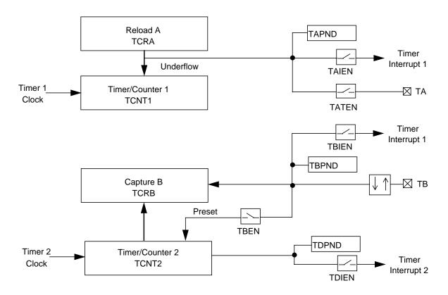
Figure 14-7. Mode 4, Input Capture and Timer
