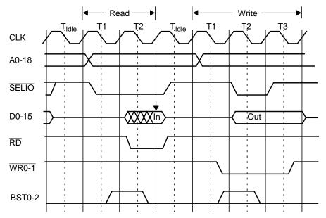
Figure 3-13. I/O Expansion Bus Cycles (BCFG.EWR = 1)
