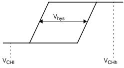
Figure 19-4. CMOS with Hysteresis Inputs
