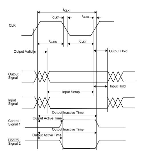
Figure 19-6. Clock Waveforms
