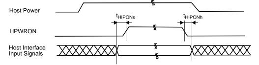
Figure 19-27. HPWRON Input Timing
