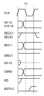
Figure 3-15. Core Bus Monitoring Bus Cycle
