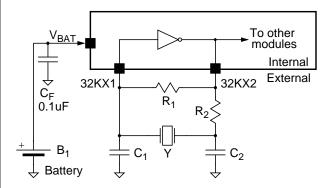
Figure 6-1. Recommended Oscillator External Circuitry
