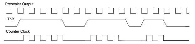
Figure 14-3. Pulse Accumulate Mode
