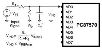
C<sub>2</sub> is an optional capacitor for noise filtering
