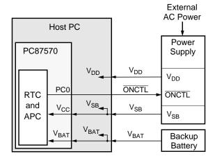
Figure 6-4. Power Supply Connections
