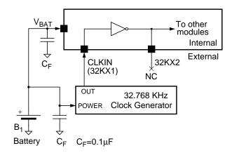
Figure 6-2. External Oscillator Connections
