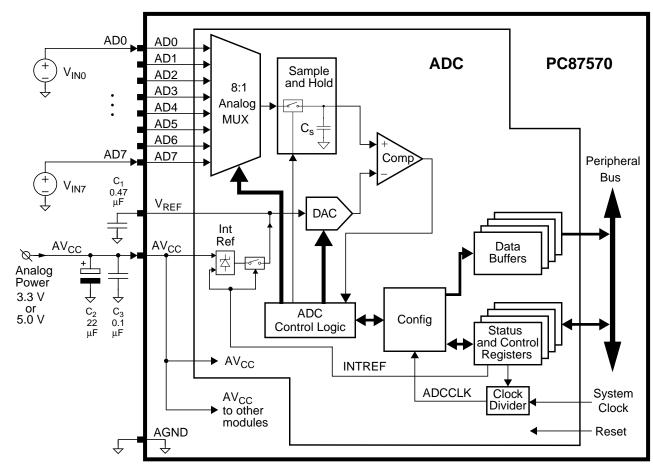
Figure 16-1. ADC Functional Diagram
