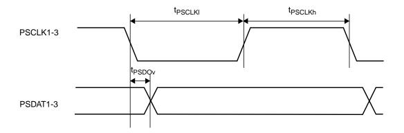
Figure 19-29. PS/2 Transmit Timing
