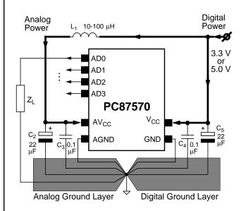
Figure 17-2. DAC Analog Power Supply Connection
