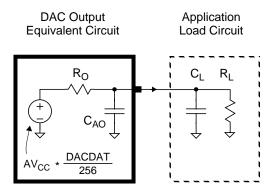
Figure 17-3. DAC Output Equivalent Circuit
