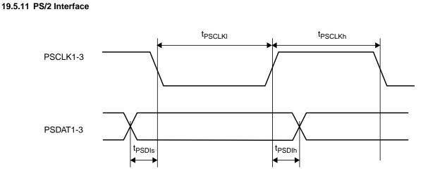
Figure 19-28. PS/2 Receive Timing
