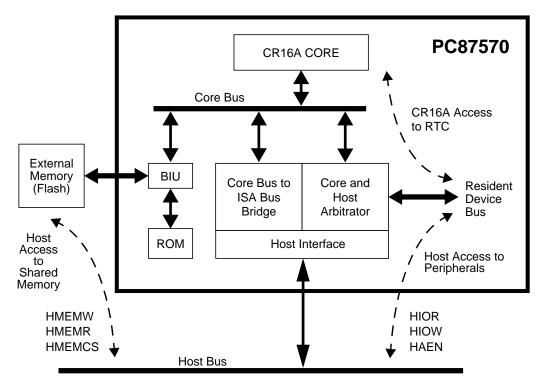
Figure 5-1. Host Bus Interface Schematic Diagram
