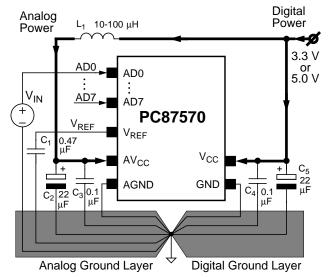
Figure 16-4. ADC Analog Power Supply Connection
