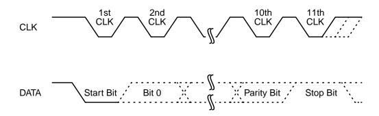
Figure 12-5. PS/2 Receive Data Byte Timing
