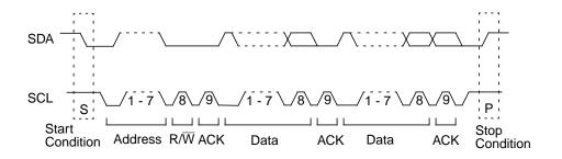
Figure 13-5. A Complete ACCESS.bus Data Transaction
