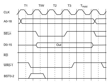
Figure 3-3. Early Write Bus Cycle with 1 Internal Wait and 1 Hold
