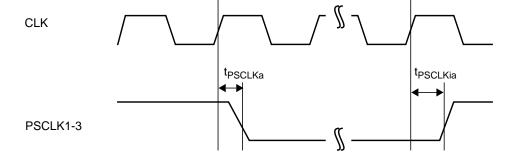
Figure 19-30. PS/2 Clock Signal Pulled Low by PC87570
