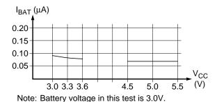
Figure 6-7. Typical Battery Current During Normal
