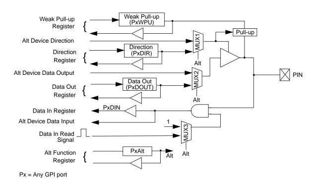
Figure 11-1. GPIO Port Schematic Diagram
