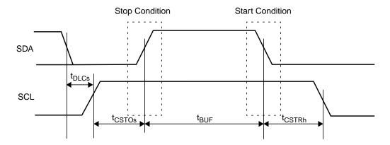
Figure 19-20. ACB Start and Stop Condition Timing
