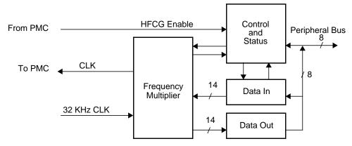
Figure 7-1. HFCG Schematic Diagram
