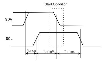
Figure 19-21. ACB Start Condition TIming
