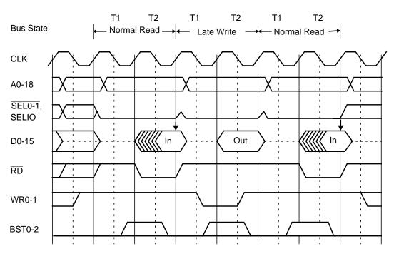
Figure 3-5. Late Write Bus Cycle Between Normal Read Bus Cycles with 0 Wait
