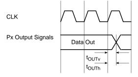
Figure 19-14. Output Signal Timing for Output and I/O Port Signals
