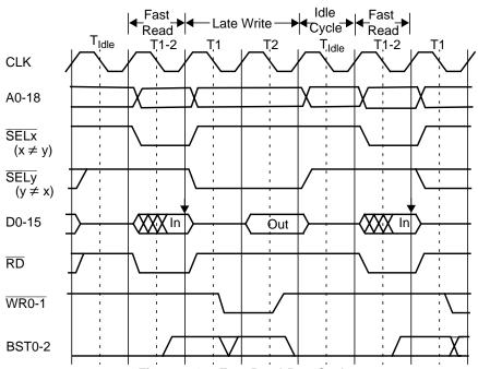
Figure 3-12. Fast Read Bus Cycle
