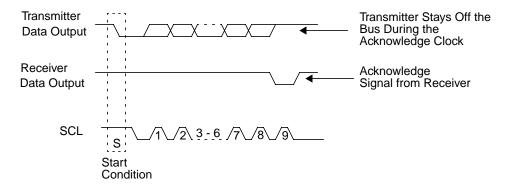
Figure 13-4. ACCESS.bus Acknowledge Cycle
