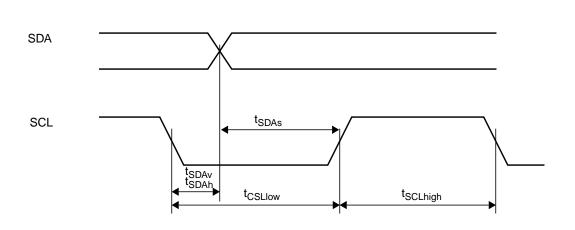
Figure 19-22. ACB Data Bit Timing
