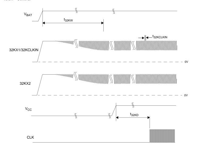
Figure 19-5. 32K Waveforms
