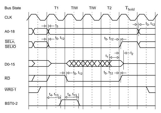
Figure 19-11. Normal Read Bus Cycle (2 Internal Waits, and 1 Hold), AC Timing
