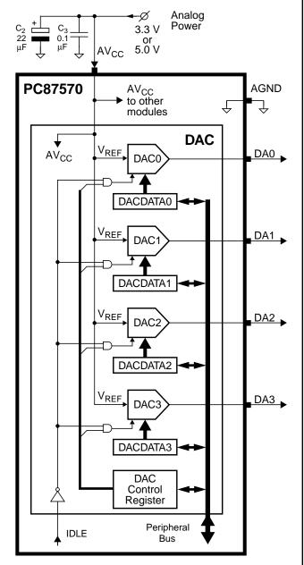
Figure 17-1. DAC Functional Diagram
