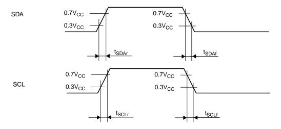
Figure 19-19. ACB Signals (SDA and SCL) Rising Time and Falling Time
