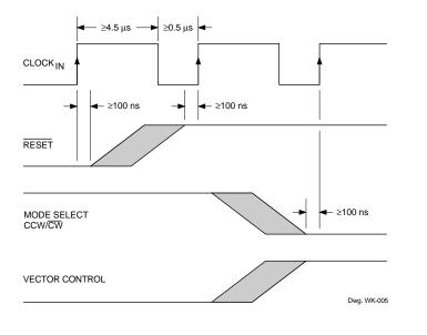
PG001M Input Signals Timing
