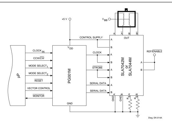
Figure 3 — Typical 'Integrated' Microstepping System
