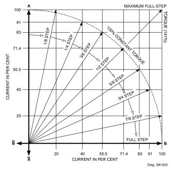
Figure 2 — Current/Displacement Vectors
