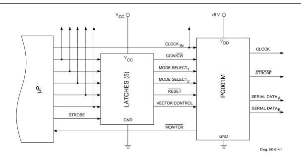
Figure 6 — A Latched Input-Bus Configuration
